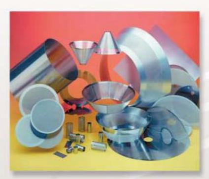
High quality Micro-Etch® products are close tolerance, precision etched perforated metal screens that have established new standards for precision, dimensional stability and discharge efficiency. They are manufactured from 300 series stainless steel in a photo chemical machining process that allows precise control of hole size and placement.
